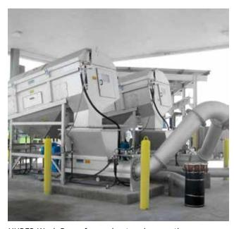
HUBER Wash Drum for washout and separation of all coarse material > 10 mm.
